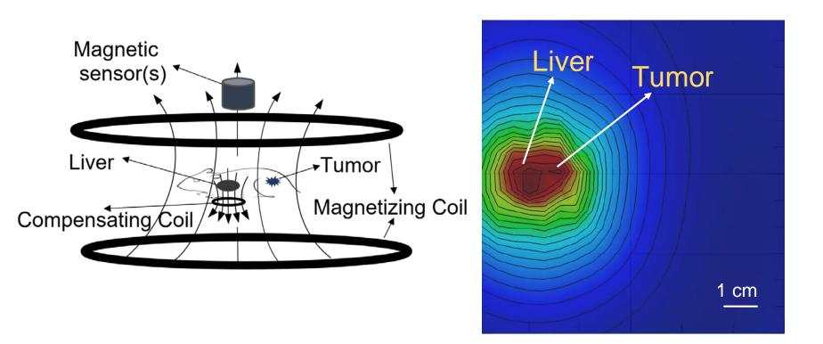
□ 6-fold reduction of the Liver signal from 3.3x10<sup>2</sup> to 0.56x10<sup>2</sup> nJ/T **Resolving a Tumor of 10% of a liver** at 2cm away from the liver □ Projected, **10-fold reduction of liver signal** with a better coil design
